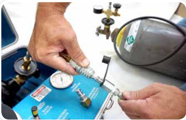
STEP 7: Align the end of the 6-Foot Filling Hose with the Model 1515D tank hose and press the two fittings together.
