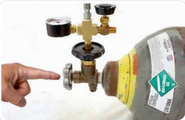
STEP 9: Ensure Supply Tank Valve is closed.
