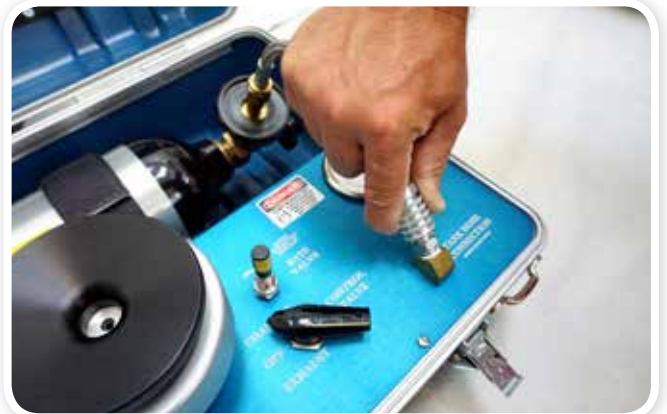
STEP 16: Connect Model 1515D Tank Hose to the instrument side. Ensure properly connected by slight tug on hose.
