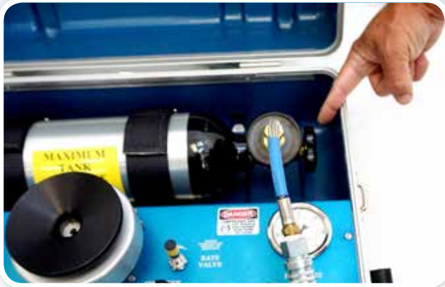
STEP II: Ensure Model 1515D Tank Valve is closed.
