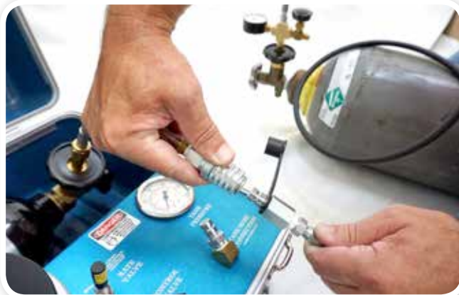
STEP 15: Disconnect 6-Foot Filling hose by pulling back on Safety Coupler on Model 1515D Tank Hose.
