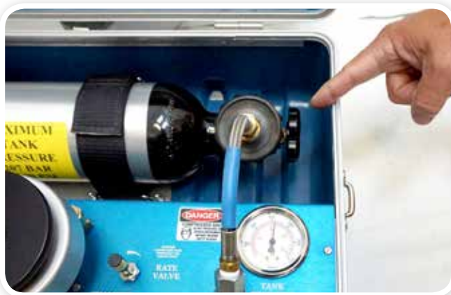
STEP 2: Close the Model 1515D Tank Valve.
