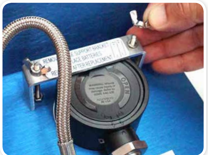
Step 6. Remove the wing nuts from gauge support bracket.
