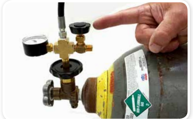
STEP 14: Close Model 1515D Tank valve. Close Supply Tank Valve. Open Exhaust Valve to release pressure from 6 Foot Filling Hose.
