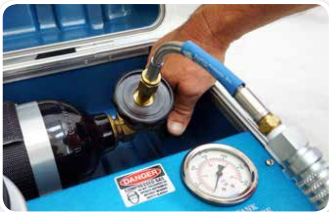
STEP 13: Open Model 1515D tank just barely. You will hear a squealing sound. As the sounds lessens, open the valve slightly more. Continue this process till valve is completely open and pressure has equalized.
