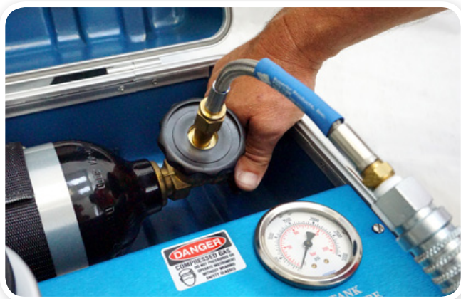
STEP 13: Open Model 615D tank just barely. You will hear a squealing sound. As the sounds lessens, open the valve slightly more. Continue this process till valve is completely open and pressure has equalized.
