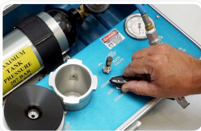
STEP 3: Ensure the chamber lid is off the chamber. Turn the control valve to "Chamber". Let all pressure escape the system.
