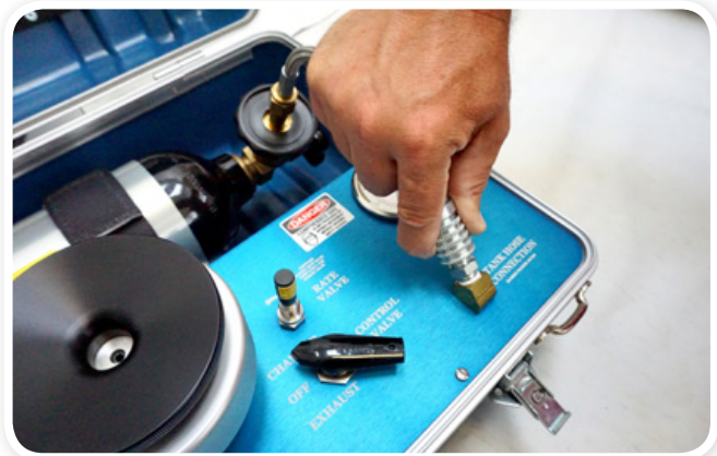
STEP 16: Connect Model 615D Tank Hose to the instrument side. Ensure properly connected by slight tug on hose.
