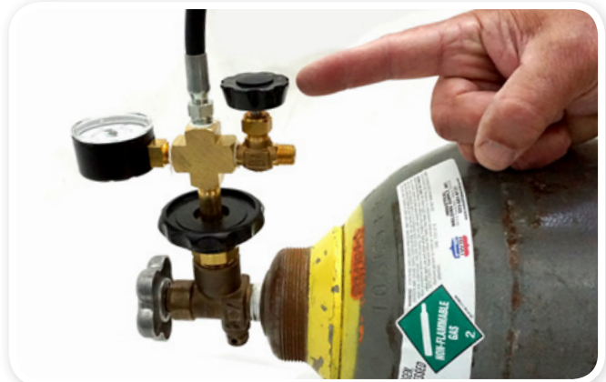
STEP 14: Close Model 615D Tank valve. Close Supply Tank Valve. Open Exhaust Valve to release pressure from 6 Foot Filling Hose.
