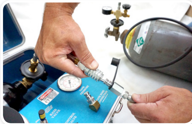
STEP 15: Disconnect 6-Foot Filling hose by pulling back on Safety Coupler on Model 615D Tank Hose.
