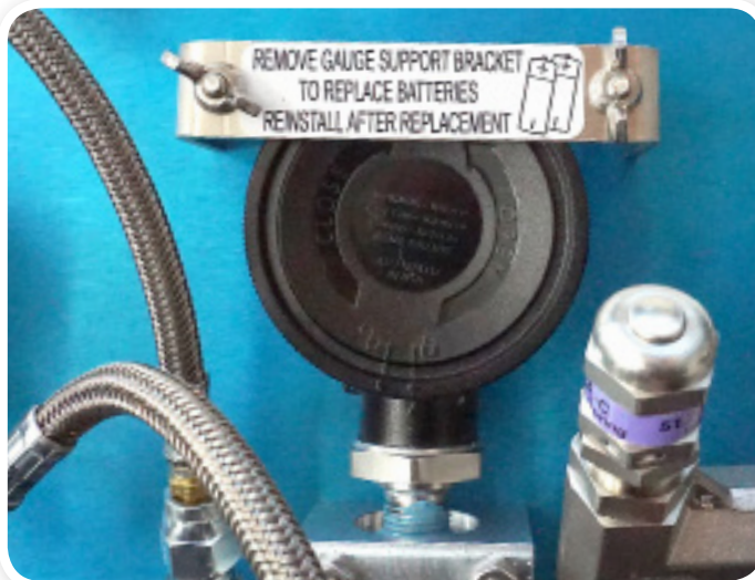
Step 4. Locate the back of the gauge and gauge support bracket.
