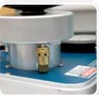
If the piston successfully cycles, the safety valve is working properly. If the piston does not cycle, refer to the maintenance section to clean the safety valve. Dirt and debris are the most common problems that result in a faulty safety valve function. Do not operate the instrument unless the safety valve is functioning properly.
