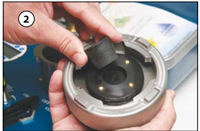
Insert a solid rubber gasket into the lid
