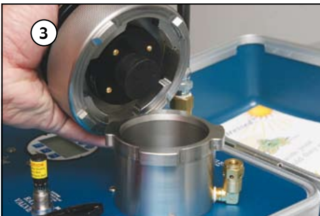
Install the lid on the chamber
